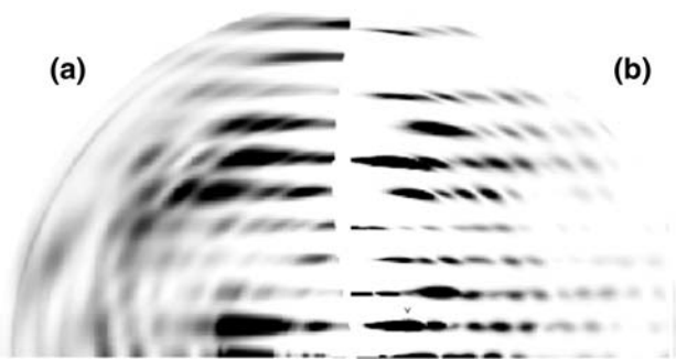
Fig. 3 X-ray fibre diffraction pattern of fd filamentous bacteriophage. A single quadrant is shown, with the fibre axis vertical. The outer edge of the diffraction pattern corresponds to about 3 Å spacing. (a) Experimentally observed diffraction pattern after background subtraction, mapped from detector space to reciprocal space and quadrant averaged (Fig. 2a of Marvin et al. 2006). (b) Calculated simulated diffraction pattern for model 2HI5. The arrow above the first layer line on b indicates a region where strong calculated intensity appears at a reciprocal space radius of R = 0.05 \text{ \AA}^{-1} , compared with R = 0.10 \text{ \AA}^{-1} on the observed diffraction pattern
